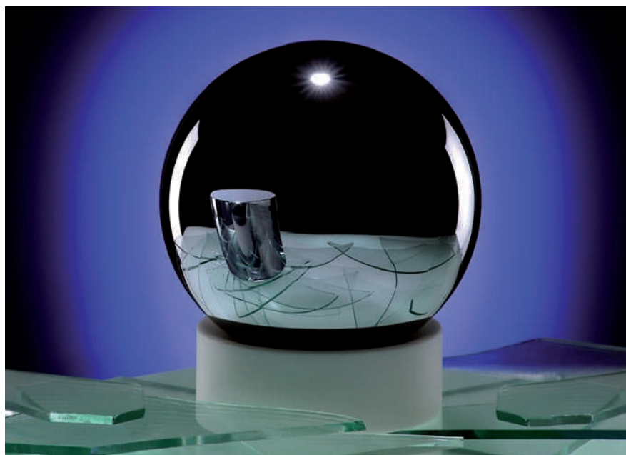
The silicon-28 sphere is the latest contender in a long weighting game.
