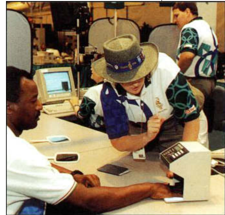
Hand geometry was used to regulate access into the residential zone of the Olympic Village.
