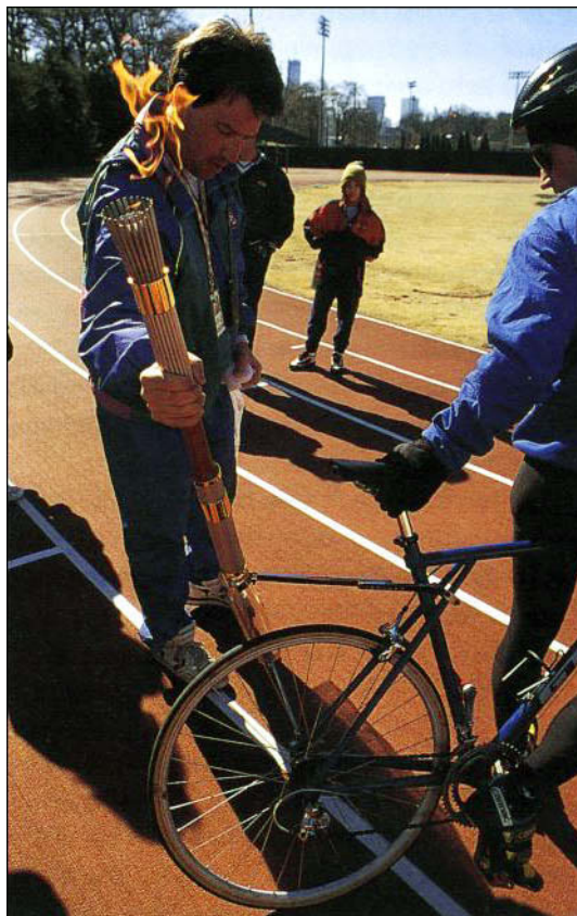
left: A bicycle torch mount is tested at the Georgia Institute of Technology.
