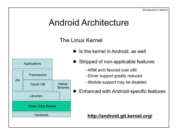
All modern operating systems are based on a **kernel**, and Android is no exception. Android uses the open source Linux Kernel as its own, albeit with some (open source) modifications.
