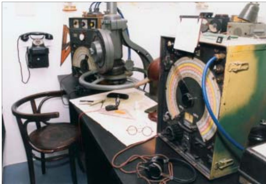
Part of the equipment of these radio detection units was a goniometer EP 2 with stationary directional equipment and a short-wave receiver Fu.H.Ec for monitoring.
