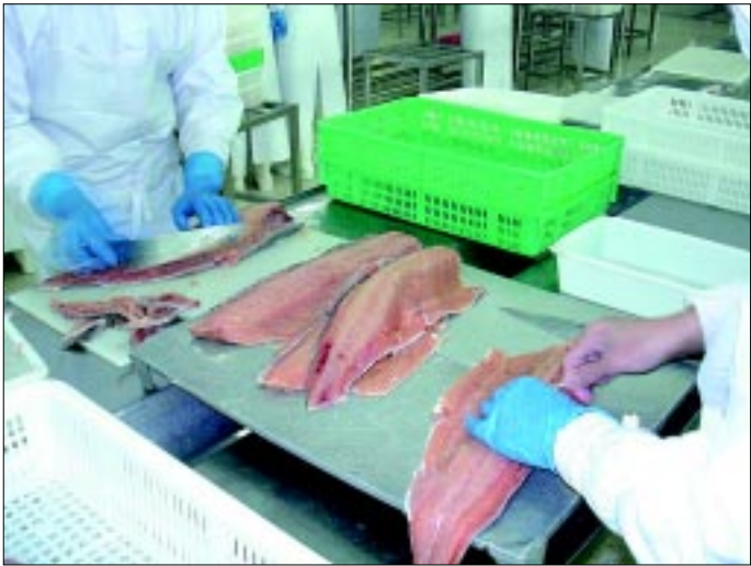
Station 2. Fillet trimming and pin bone removal. Pin bone removal is done with the use of tweezers.
