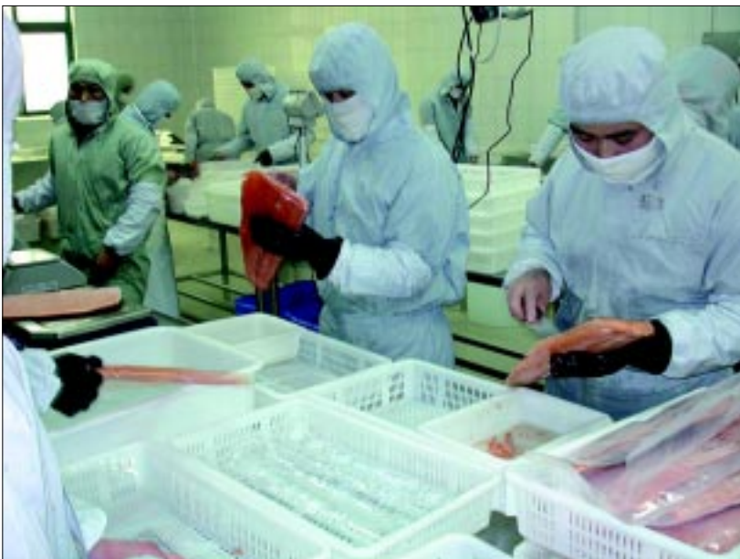
Station 6. Post-freezer trimming. Any ice pieces attached to the frozen fillet are tapped off with a knife to improve appearance. These fillets will be passed through a metal detector and then packaged according to client specifications.
