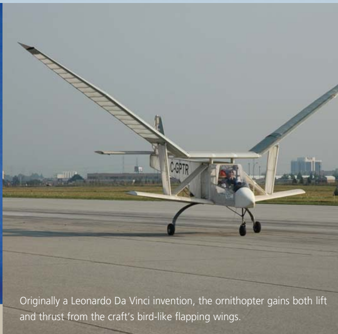
Each of the ornithopter's wings consists of three hinged panels supported by centre pylons and outboard vertical links.
