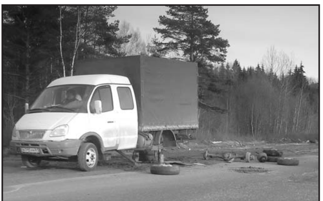
Untold damage to the economy. This truck's rear axle spills out onto the road because its driver didn't follow the posted speed limit.
