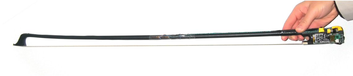
Figure 2.3: The original Hyperbow for violin, which was used in the performances of Toy Symphony , was adapted for use with cello. Two of these Hyperbows for cello were built for the ongoing collaboration with the Royal Academy of Music.
