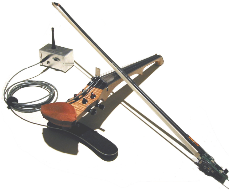
Figure 2.1: The Hyperbow sensing system that was developed for the Toy Symphony project was installed on a Jensen electric violin and a CodaBow® Conservatory™ carbon fiber violin bow. The system was optimized to be lightweight and compact and relied on minimal external electronics.
