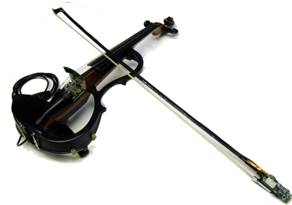
Figure 3.8: The final hardware implementation for the playable measurement system for violin bowing was installed on a Yamaha SV-200 Silent Violin and a CodaBow® Conservatory™ carbon fiber violin bow. The bow remained wireless, while the violin electronics used one USB cable for both data communication and power (as well as one audio cable not pictured).
