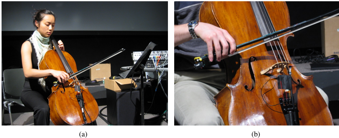
Figure 2.4: (a) Royal Academy of Music masters student Shu-Wei Tseng performing Patrick Nunn’s Gaia Sketches on acoustic cello and Hyperbow. (b) Closeup of Hyperbow and acoustic cello. Here, the placement of the antenna for the bow position sensor has been improvised by the composers and cellists from RAM.
