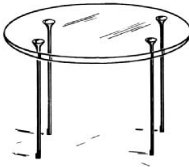
Fig. 6.5 A lightweight table with slender cylindrical legs. Lightness and slenderness are independent design goals, both constrained by the requirement that the legs must not buckle when the table is loaded. The best choice is a material with high values of both E^{1/2}/\rho and E .
