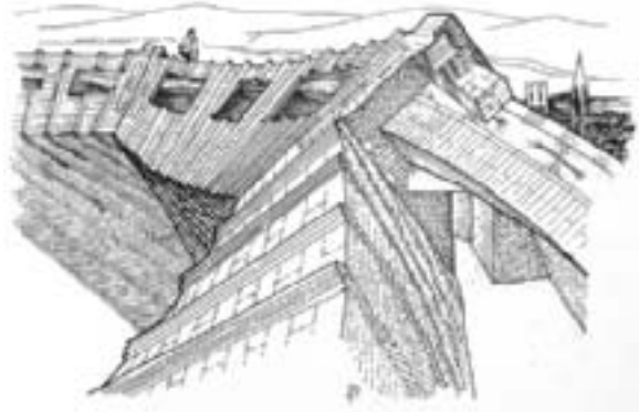
Fig. 17: Duomo, Florence. General view and construction detail. Brunelleschi. (Gärtner; Mark)
