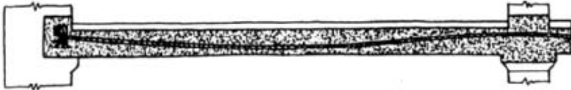
Fig. 3: First reinforced concrete beam patent, Wilkinson, 1854. Wilkinson used wire rope positioned to resist the principal tensions in the floor. (Mainstone 1 )
