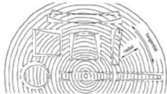
Fig. 45: Shrinkage characteristics of different cuts of wood from trunk. (Perry 2 )
