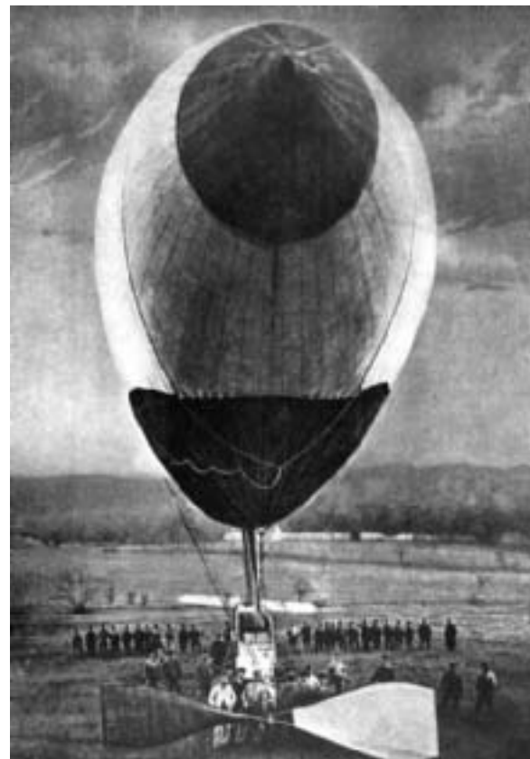
Fig. 2: La France , first dirigible airship. Non-rigid type. Charles Renard, 1885. (Knäusel)
