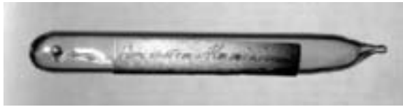
Fig. 12: Test tube holding aluminum particles reduced by Friedrich Wöhler, 1845. (Nichols)
