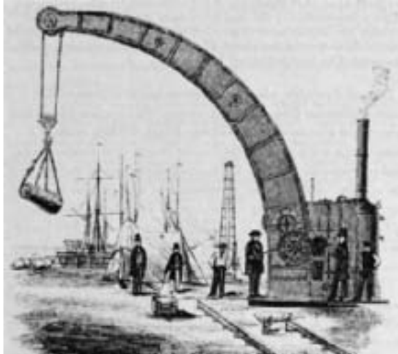
Fig. 78: Fairbairn type crane with tubular structure. (Rosenberg and Vincenti)
