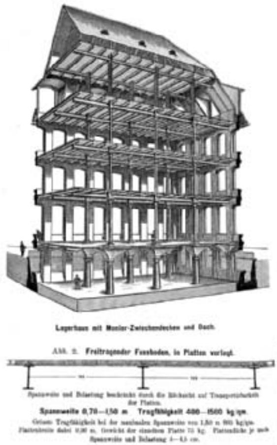
Fig. 23: Monier Composite System (Waysys)
