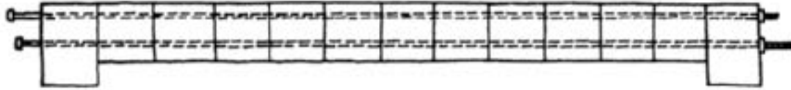
Fig. 2: Prestressed, reinforced masonry beam, Pope, 1811. (Pope)
