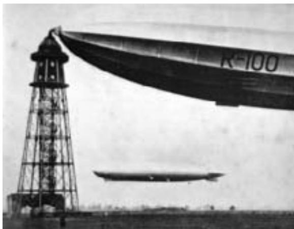
Fig. 11: The mooring mast, a British invention, allows the airship to turn 360° with the wind while moored. (Hartcup)
