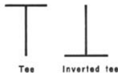
Fig. 31: Orientation of cast-iron T-sections tested by Hodgkinson showing that the inverted-T is stronger by a ratio of 1:4. (Jewett)
