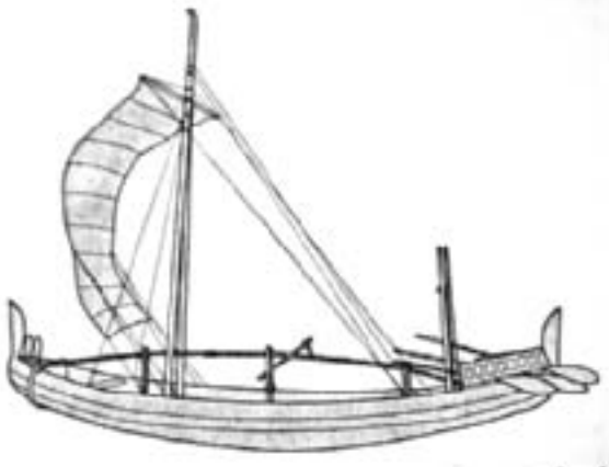
Fig. 13: Egyptian sea-going vessel made of wood modeled after Nile boats made of bundled reeds. The wooden ship retains the vertical ornaments at stem and stern characteristic of the reed-built boats. The wooden planks would have been short and poorly fastened therefore this ship retains the traditional Egyptian hogging-truss, c.2,500 BC. (Gordon)
