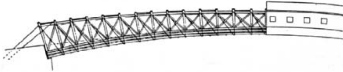
Fig. 11: The "Colossus," an arched through-truss with a single span of 103.6 m (340 ft) built at Philadelphia, Wernwag, 1813. (James 2 )
