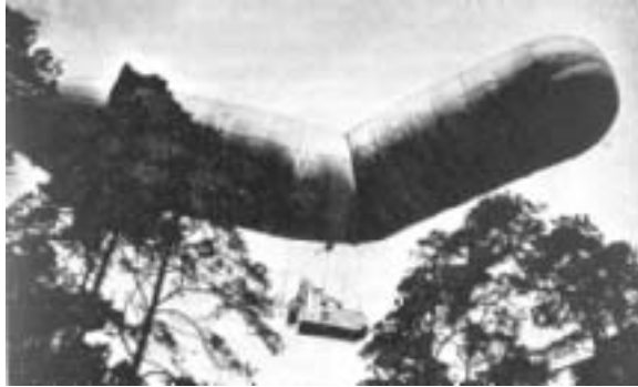
Fig. 5: Buckled envelope of a non-rigid due to moment stress in the gas envelope. German aeronaut August von Parseval designed the pictured ship. (Knäusel)
