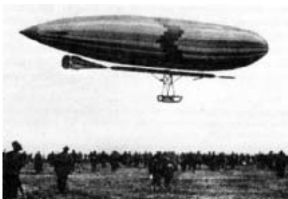
Fig. 7: A semi-rigid type airship with rigid spine on underside of envelope. Shown is a German Gross-Basenach airship. (Knäusel)
