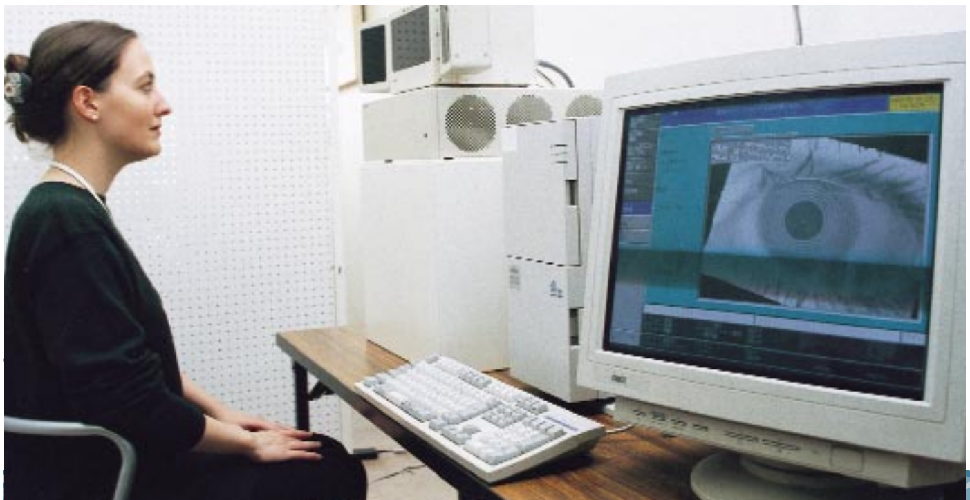
An iris scan system was used to guard the biathlon rifle storage facility at the Olympic Village.
