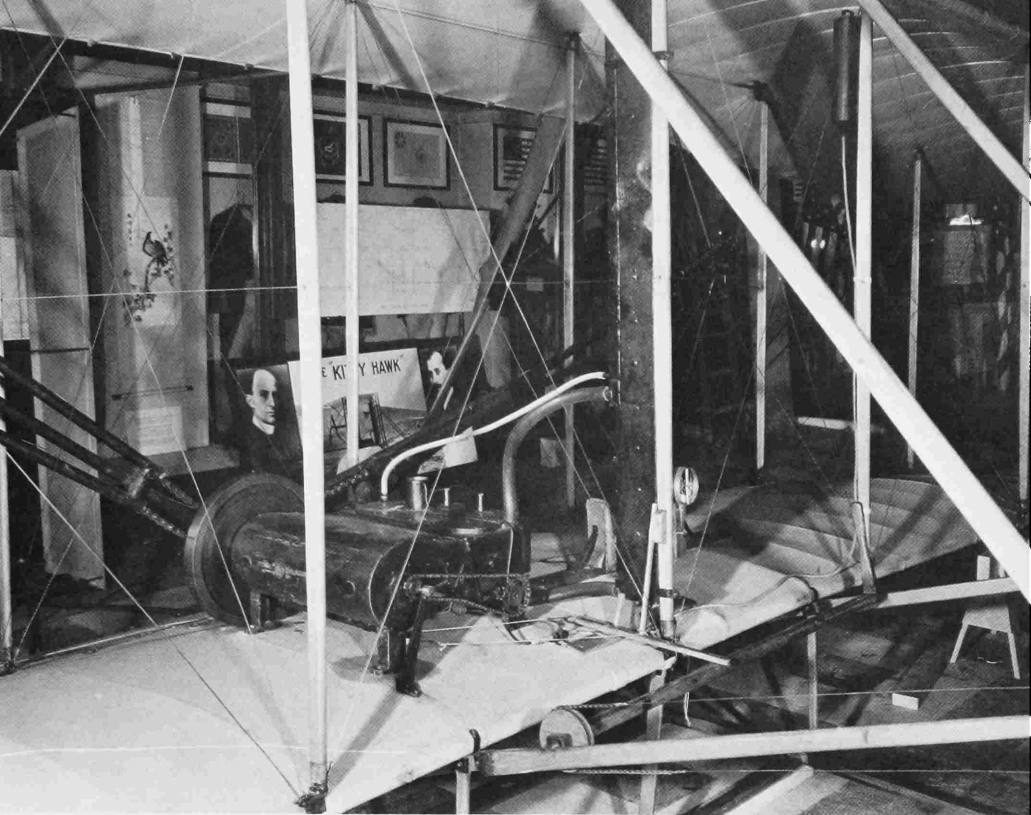
Figure 3.—First flight engine, 1903, installed in the Kitty Hawk airplane, as exhibited in the Science Museum. (Photo courtesy the Science Museum, London.)
