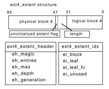
Figure 1: Ext4 extents, header and index structures
