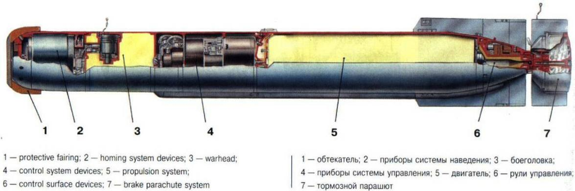
*Figure 13. Russian APR-2E rocket torpedo*
