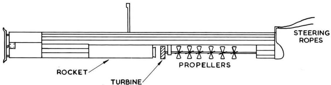
*Figure 3. The Berdan Rocket Torpedo, c1885*
