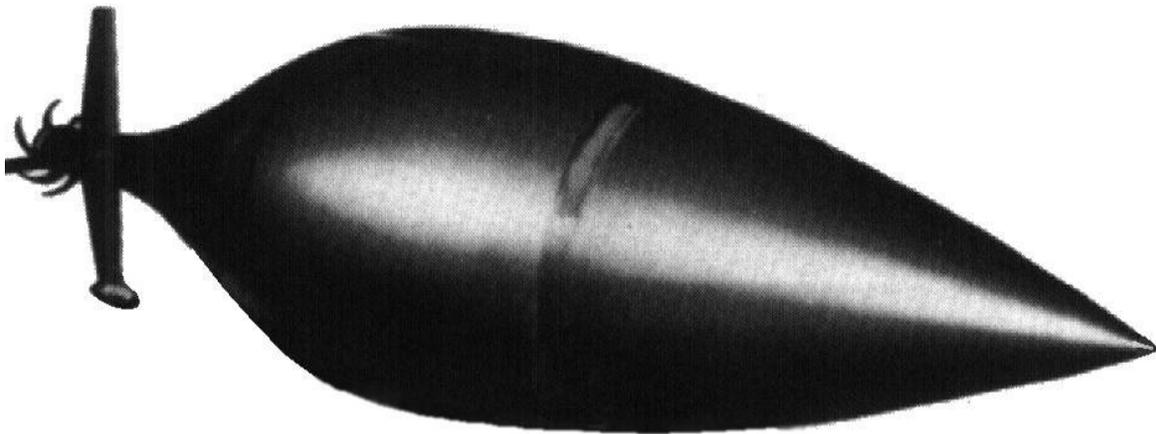
*Figure 12. A US laminar-flow body*
