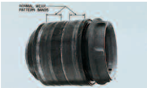
Figure 13 Normal Wear Bands on Outer Ring (Bearing Cup)
