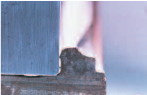
Figure 19 Gaging Adapter Thrust Shoulder Wear
