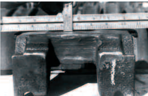
Figure 21 Adapter with Hollow Wear Caused by Frame Roof Liner
