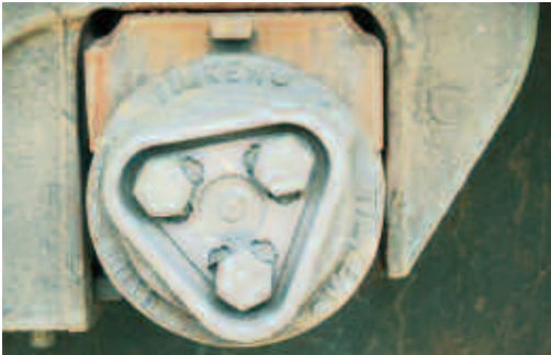
Figure 15 Adapter in Truck Frame Pedestal
