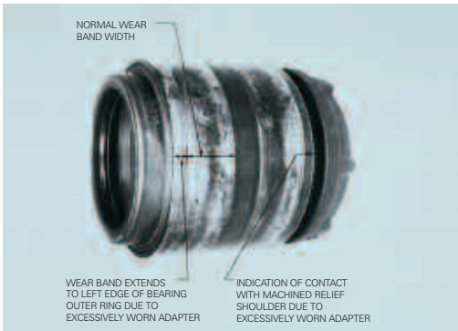
Figure 14 Wear Patterns on Outer Ring (Bearing Cup) Caused by Excessively Worn Adapter
