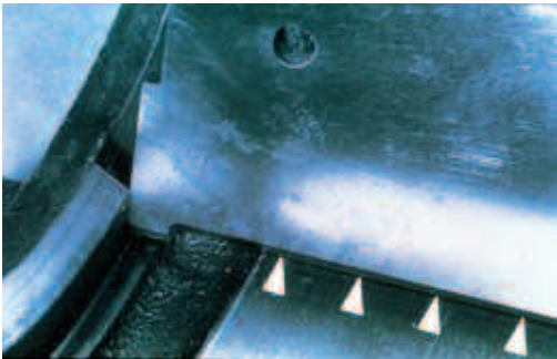
Figure 16. Gaging Adapter Bearing Seat Pad Wear. Edge of Gage Contacting Bearing Seat Pad - OK
