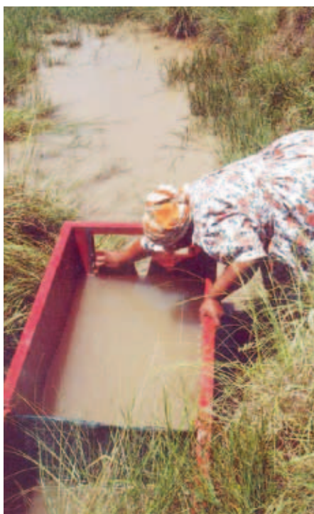
Measuring streamflows from ‘portable’ weir
