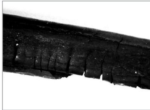
Extreme thermal stress on an O-ring
