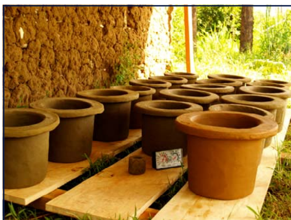
The ceramic filter, CeraMaji, filters over 99.99% of bacteria and parasite implicated in gastrointestinal diseases and diarrhea.
