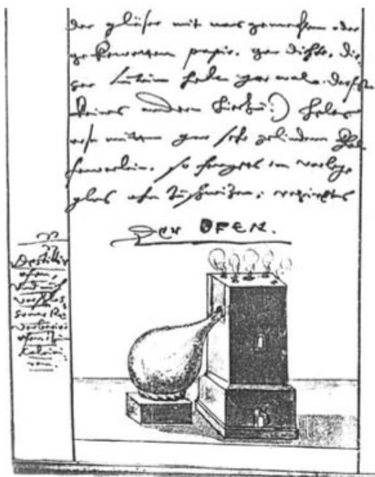
Figure 9: The furnace and recipient, from the Consilium Philosophicum Practicum , f. 16 verso (Khunrath’s autograph).
