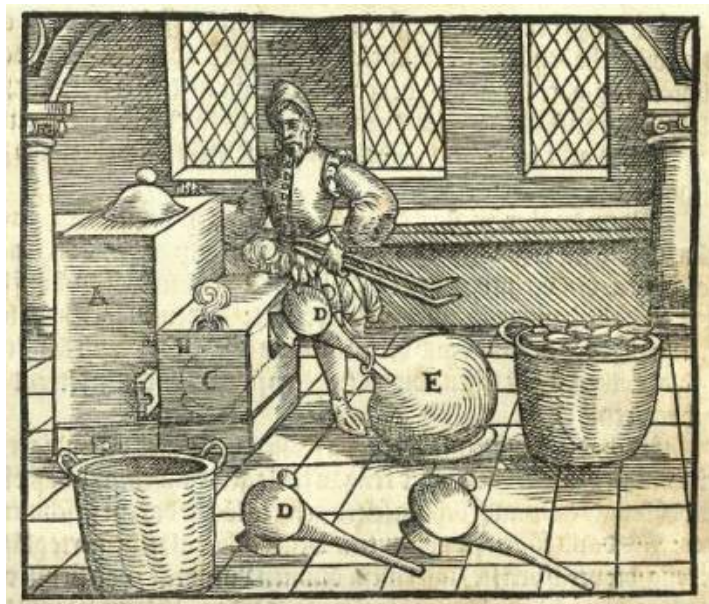
Figure 6: The distillation of aqua regia , from Lazarus Ercker's Aula Subterranea (1580). With permission of the Bayerische Staatsbibliothek, Munich.
