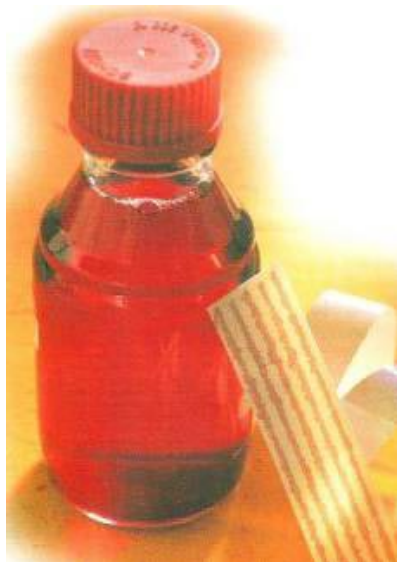
Figure 12: A gold sol manufactured with trisodium citrate. With permission of Professor Basab Chaudhuri, University of Calcutta.
