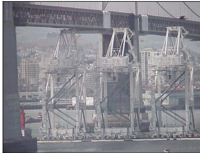
Crane barge with just enough bridge clearance during transit
