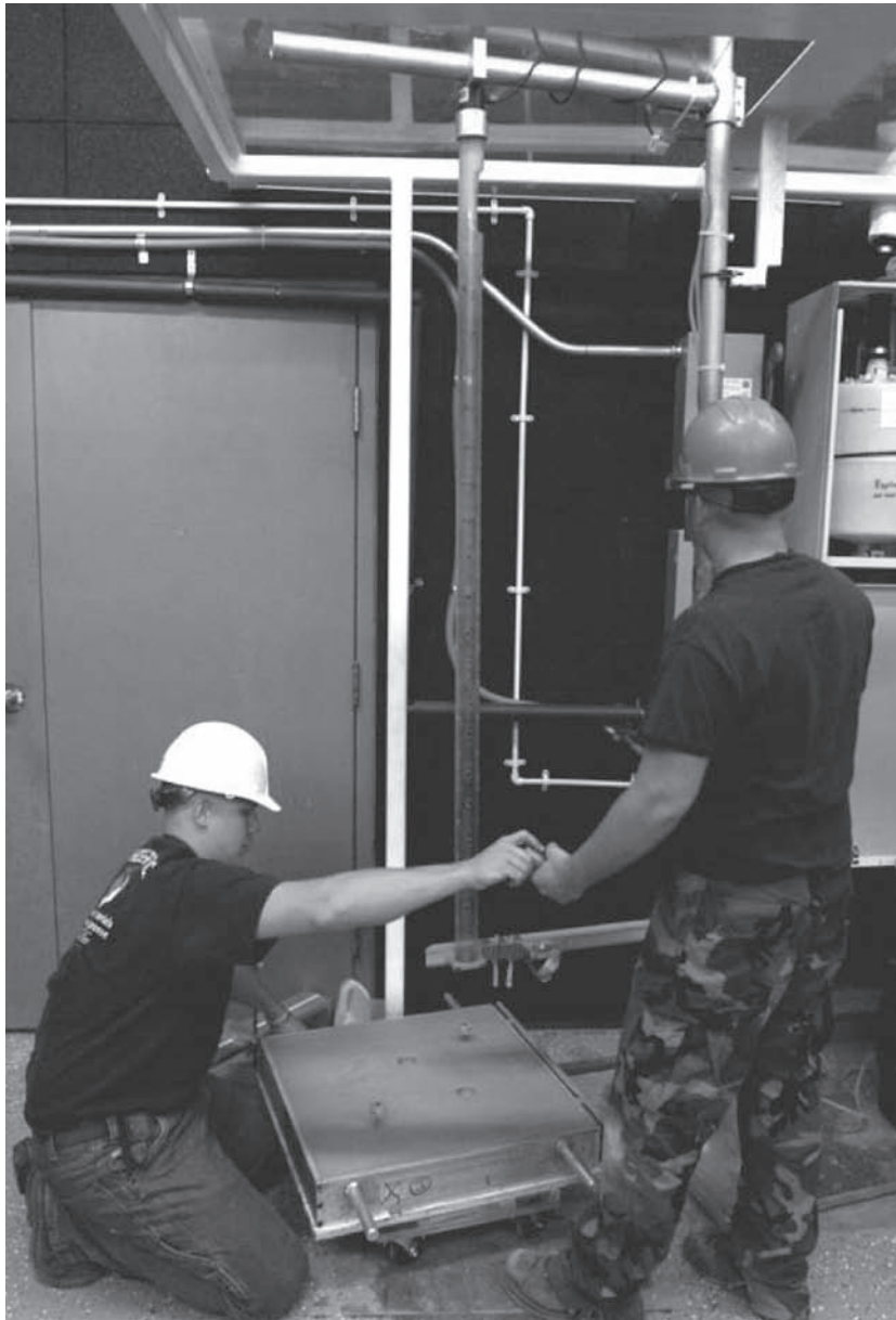
Figure 3: Clay Being Calibrated with Pre-Test Drops
