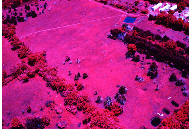
Figure 18. Color-infrared photograph of the tract immediately north of the central building complex; view toward southeast. In this type of image, photosynthetically active (green) vegetation appears in red and pink colors. Numerous dead trees are revealed by bluish gray color of bare limbs. Image acquired in late spring, June 2003.
