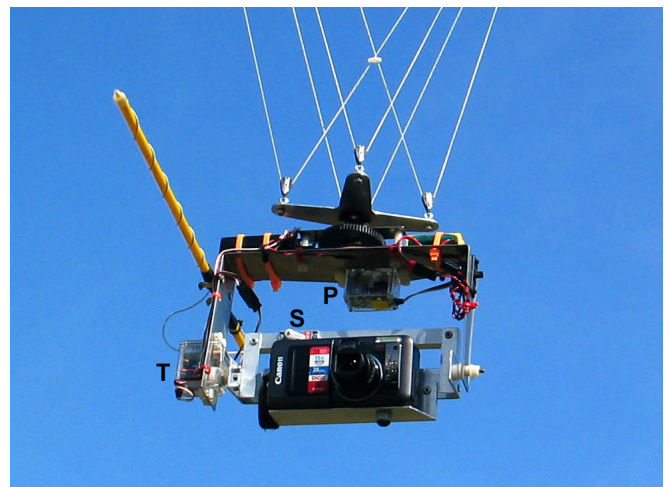
Figure 4. Small-format aerial photography camera rig for use with a kite or blimp. Seven megapixel Canon S70 digital camera is operated in a fast-shutter mode to minimize motion effects. Titanium frame holds servos for tilting (T) and panning (P), and a microservo on the aluminium cradle triggers the shutter button (S). Servos are controlled via radio signals from the ground.
