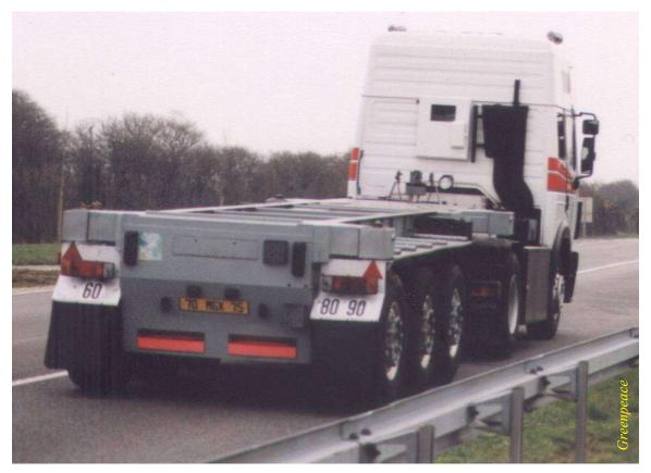
Photo 3: French plutonium transport trailer without ISO container
