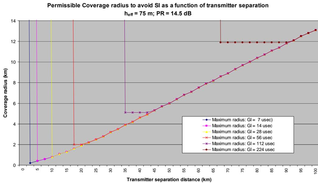
Figure 5.1: Coverage radius to avoid self-interference.
