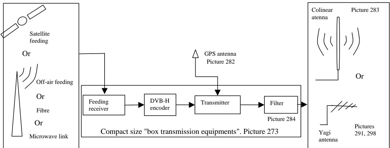
Figure A2.1: Simplified block diagram of a typical site of the LPDN topology
