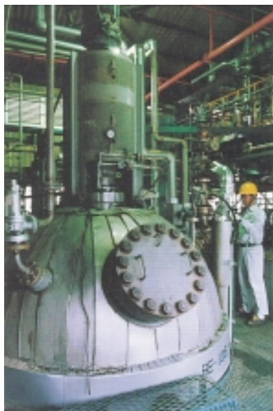
Figure 15. A large-scale BINAP–Ru catalyzed hydrogenation at Takasago International Co.
