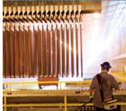
Copper cathode production at Morenci, Arizona
