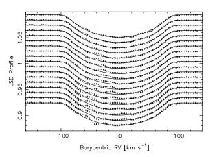
**Figure 3.** Least-squares deconvolved profiles of HD 15082 during the planetary transit of 2009 December 08 observed at the NOT. Data are shown as points with error bars. The limb-darkened stellar rotation profile is shown as a solid line. Time increases vertically. The planet signature is the positive bump that migrates from  $v \simeq 5 \, \mathrm{km \ s^{-1}}$  in the first (bottom) profile to  $v \simeq -40 \, \mathrm{km \ s^{-1}}$  in the last (top) profile shown.
