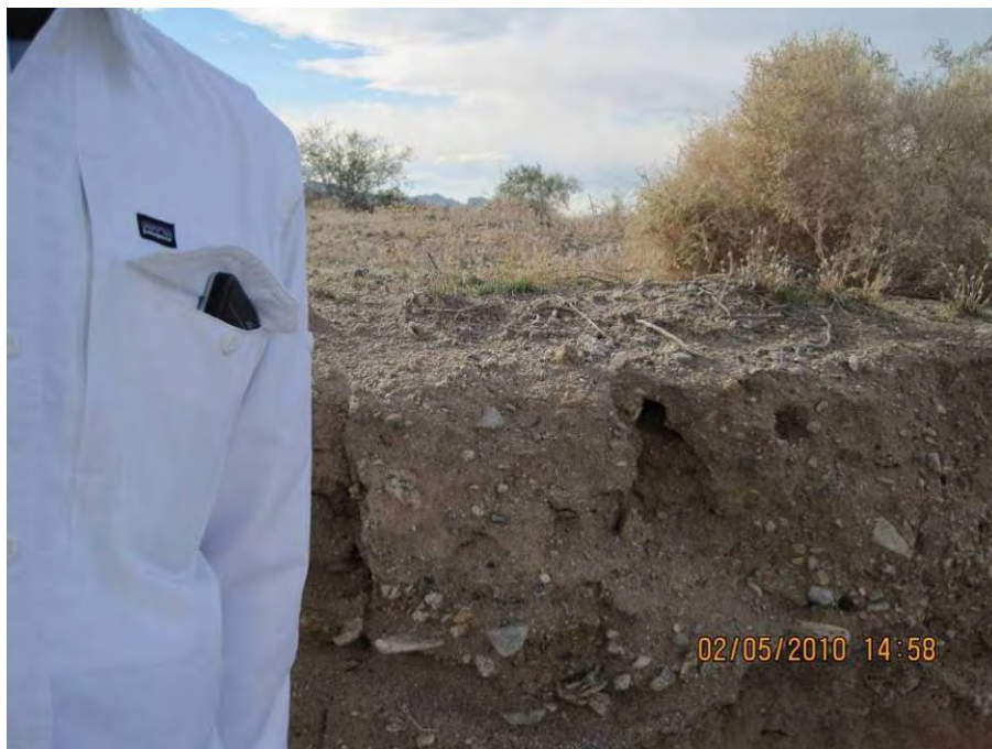
Figure 22. Channel bank is 4 feet high. Gravel in the fan provides armor that stabilizes the channel.
