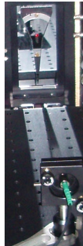
Figure 2: Launching the LFC into UHRF in the pre-slit area. The mode-filtered LFC light at 780 nm is delivered via single-mode optical fibre (black, insulated cable with green, mounted end plug) to the pre-slit entrance of UHRF and launched in free space through a diffuser (not shown) onto the slit (reflective area with decker jaws), greatly over(under)-filling it in the spectral(spatial) direction. The red laser spot visible in this photograph is not the LFC, which was at 780 nm, but a diode laser at 638 nm fed by the optical fibre from the LFC set-up bench for alignment purposes.
