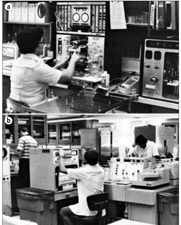
Figure 8. Laboratory automation in the 1970s: (a) a Coulter counter to perform complete blood counts; (b) an SMA-6 machine to measure blood levels of sugar, urea nitrogen, sodium, potassium, carbon dioxide, and chloride.
