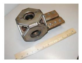
**Figure 9.** Pulsed compression device PZLx-1 built to study hydromagnetic stability of polyhedral field
