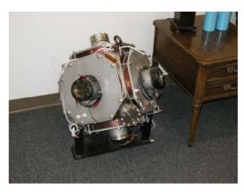
**Figure 8.** PXL-1 reactor for studying the electron cyclotron resonance
