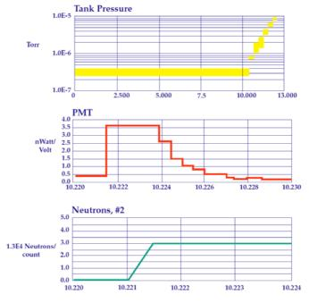
Figure 18. Neutrons obtained during WB-6 experimentation
