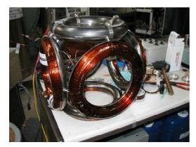
Figure 11. Construction detail of WB-6 coils
