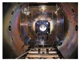
**Figure 13.** WB-6 assembled. WB-6 achieved a record of DD fusions (1E9 fus/sec) at a potencial well of 10 KV
