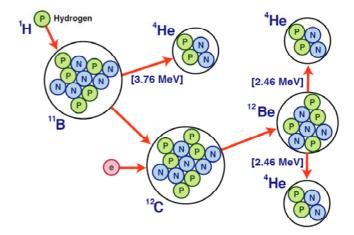
Figure 3. Aneutronic fusion:  $p + B11 \rightarrow 3 \text{ He4}$
