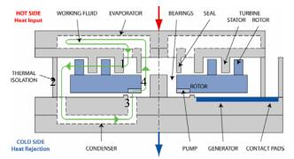
**Figure 1** - Cross-section schematic of micro steam-turbine power plant-on-a-chip. Constructed from 5 silicon wafers that are deep reactive ion etched and bonded to integrate the components on a single chip.
