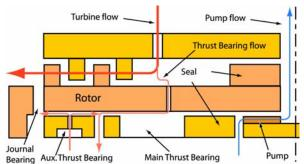
**Figure 2** - Cross-section schematic showing the main and secondary flow paths. Axial balance is created by bleeding some of the turbine inlet steam under the disk, with the pressure controlled by the outer bearing.
