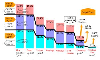
Figure 3 - Predicted performance of the Micro Steam Turbine Power Plant-on-a-chip for three configurations. Bars illustrate the reduction in power as the various sources of loss in the system are incrementally added, from left to right (water 24mg/s,  $P_{max}$ =0.6 MPa).
