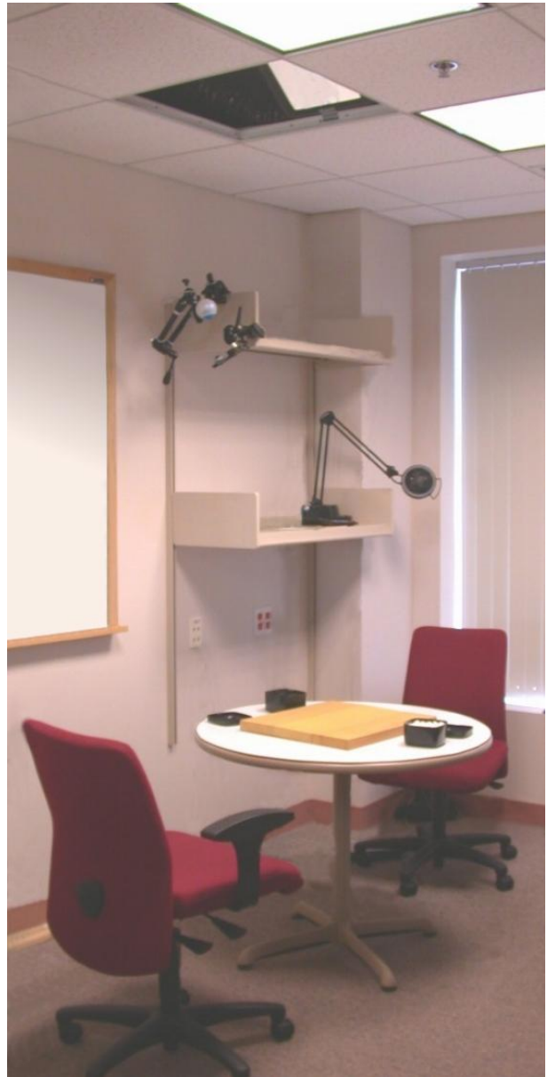
Figure 2: The system we implemented is governed by the design philosophies of parsimony and transparency articulated above. The system itself consists of a light-table comprised of a video camera and projector situated above a go board on normal table. The system projects visual annotations that form a superset of the traditional board functionality. The vision system explicitly supports our design philosophy by accommodating the traditional style of game play.
