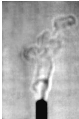
Fig. 2 Sunlight shadowgram of the convective plume from a candle flame (photo by author)
