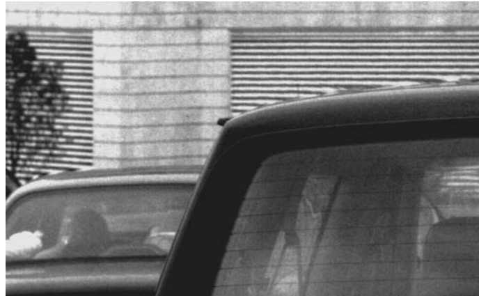
Fig. 5 Thermal boundary layer on hot car roof, seen by distortion of background grid pattern (photo by author).
