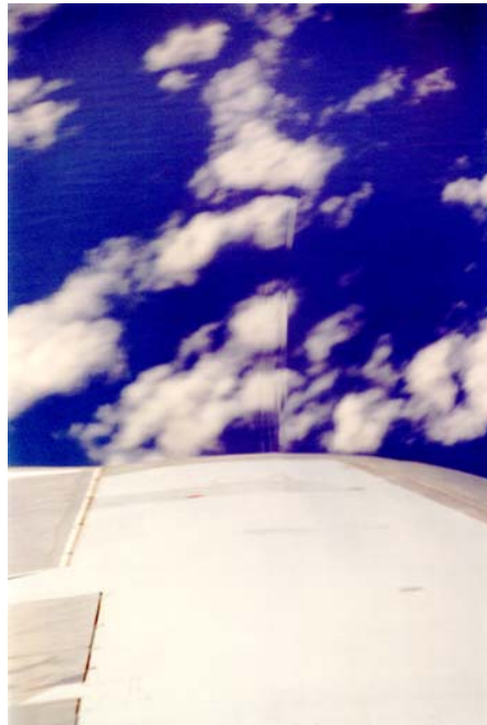
Fig. 9 Shock wave on L-1011 wing (US Govt. photo by Carla Thomas, NASA Dryden Research Center).
