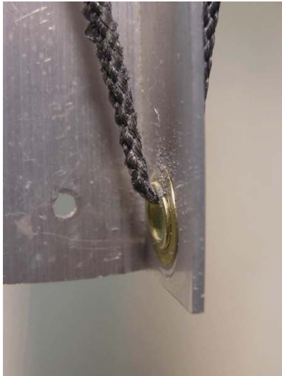
Photos 11 A and B Details of Grommet with Boot Lace
