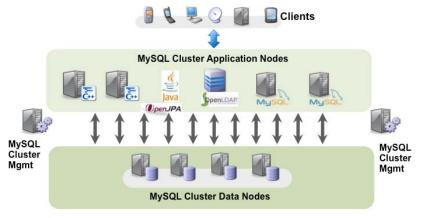
Figure 1. The MySQL Cluster architecture has been designed for five 9s availability and delivers massive read/write scalability.
