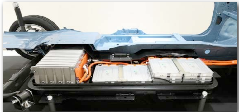
Source: Nissan. Depicting Nissan Leaf's Battery Configuration
