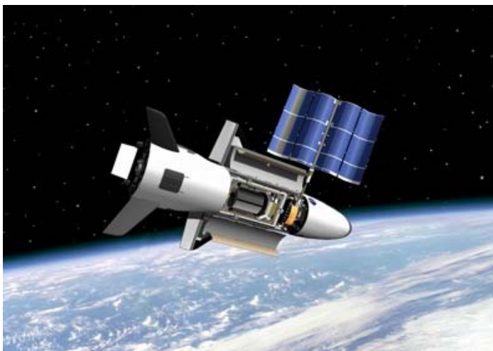
Artist's rendition of how the X-37B will deploy on orbit, including the solar panels used for electrical power
