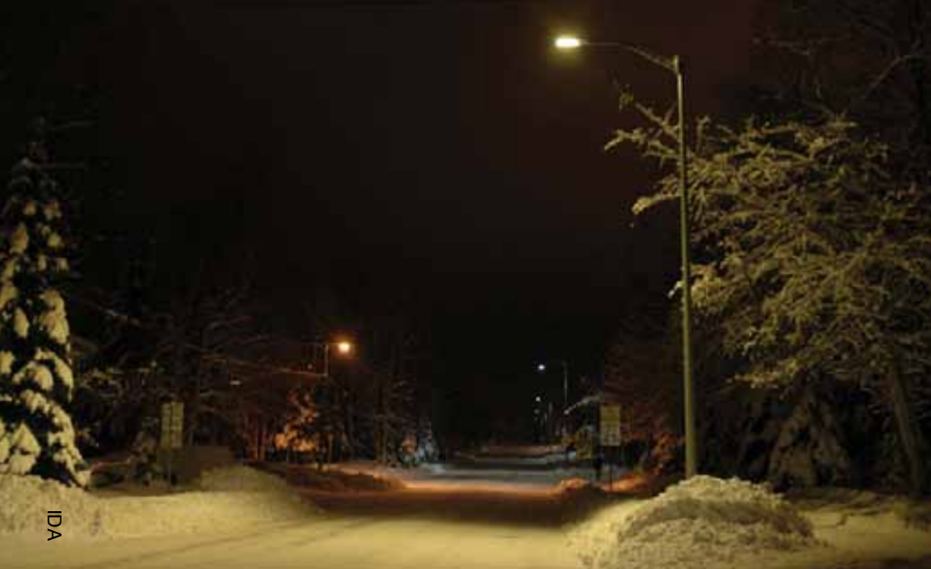
This test street in Anchorage, Alaska, USA compares the quality of light from warm, low CCT LEDs (right foreground), high pressure sodium vapor (left middle) and cool, high CCT LEDs (right background). The residents of this street preferred the warm LEDs in the foreground.
