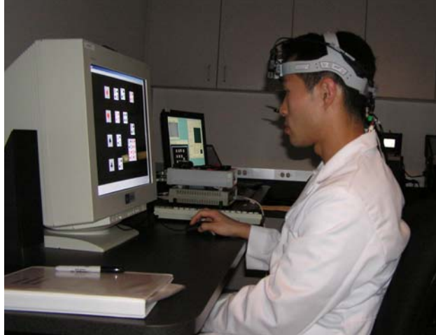
Figure 2.13. A member of the experimental team demonstrates the desktop computer experimental environment, wearing the head mounted eye tracker
