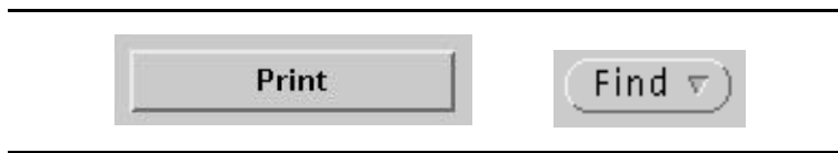
Figure 2.6 Two buttons, the left one is Motif style, the right one Open Look.
