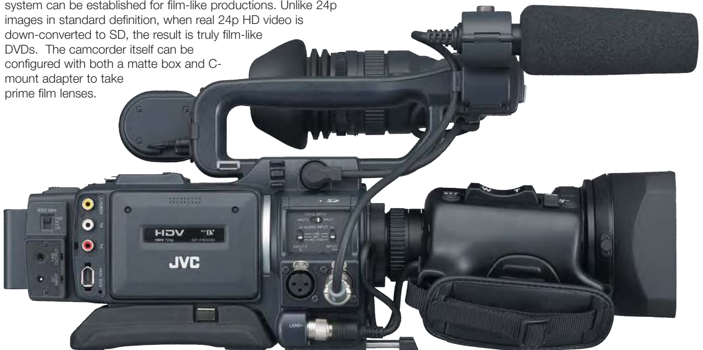
This view shows the twin XLR audio connectors and the SD memory card slot.
